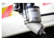
HTN bin washing nozzle washes whole bin in 15s run
